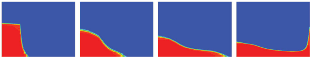
Figure 13. Numerical production of entropy at time 0.1, 0.2, 0.3, and 0.4 s (blue, zero; red, negative values).
