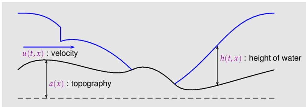
FIGURE 4. Description of the shallow-water model.
